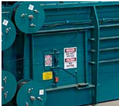
Lower ram chassis inspection door for easy maintenance access.
